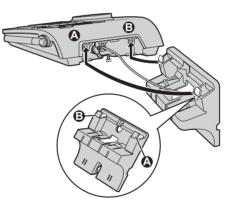
**3** Adjust the adaptor to hold the base unit, then push it in the direction of the arrow until it clicks into place.
